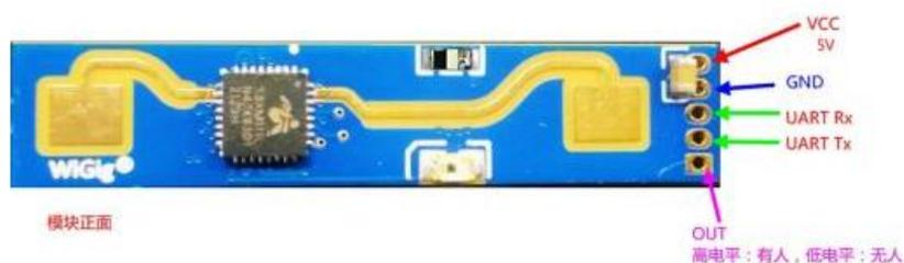
Figure 6 Module pin definition diagram
