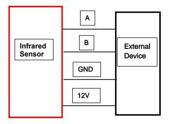
Shanghai GASIM intelligent network type intelligent infrared can read and modify internal registers through 485 communication to achieve remote monitoring and output control. Communication protocol refer to MODBUS RTU communication format. Serial port setting: baud rate "9600", parity bit "none", data bit "8", stop bit "1", data is accessed by master-slave query mode, sensor is slave there is only one node on the bus sending data. Note
