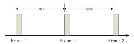
(4) Sending broadcasting data only, not for connection. Master device doesn't need to send data to other sensors.
