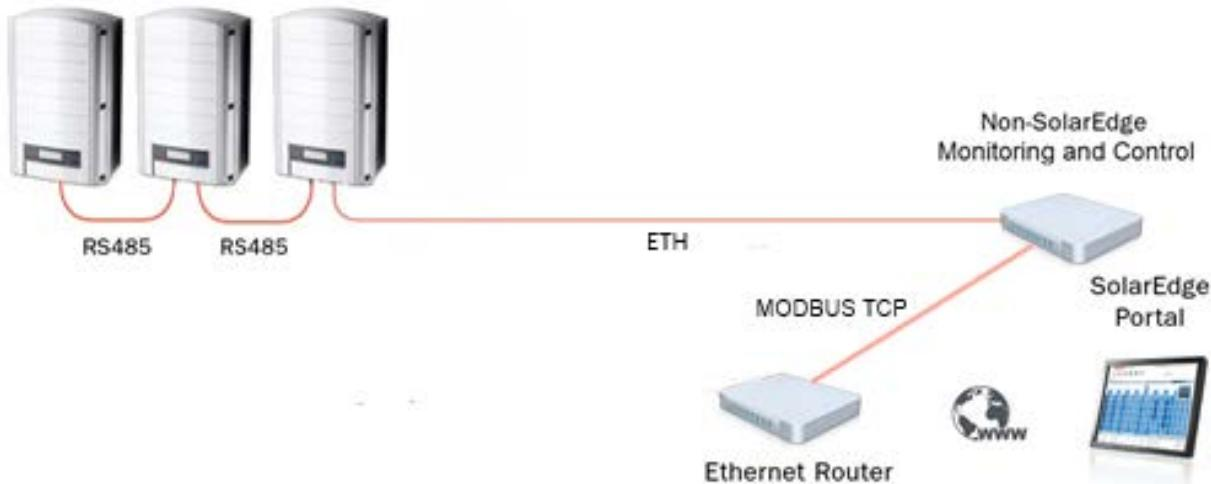
Connection to SolarEdge monitoring portal and to a non-SolarEdge monitoring device using SolarEdge Control and Communication Gateway
