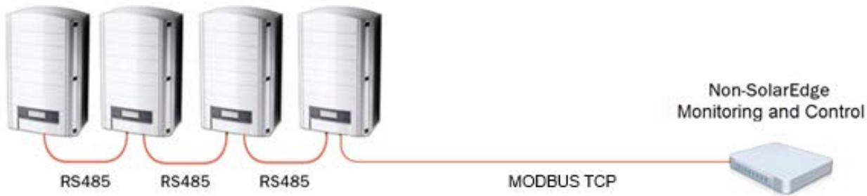
Connection to the SolarEdge monitoring portal and to a non-SolarEdge monitoring device
